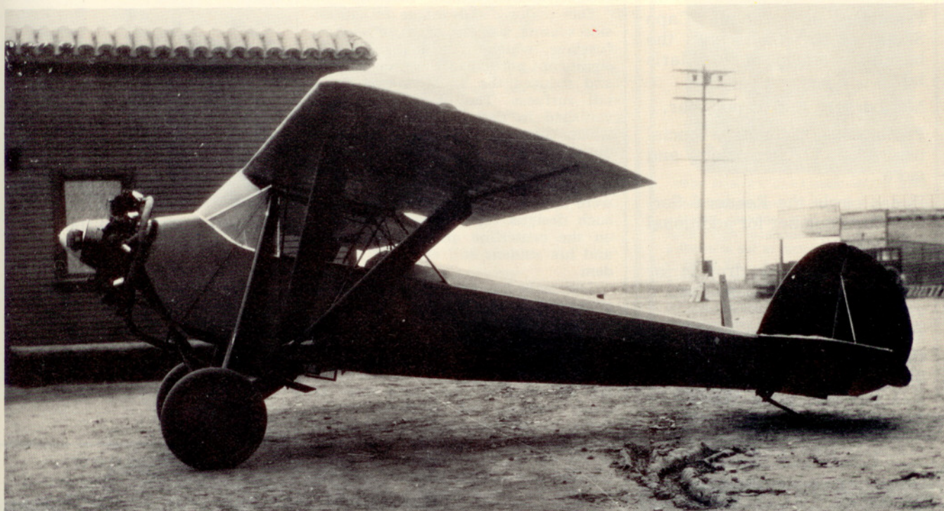
This early Mono Aircraft Monoprep was fitted with 1928-style Monocoupe landing gear and a curved center windshield panel. Compare fin and rudder shapes with later models in other photos.
