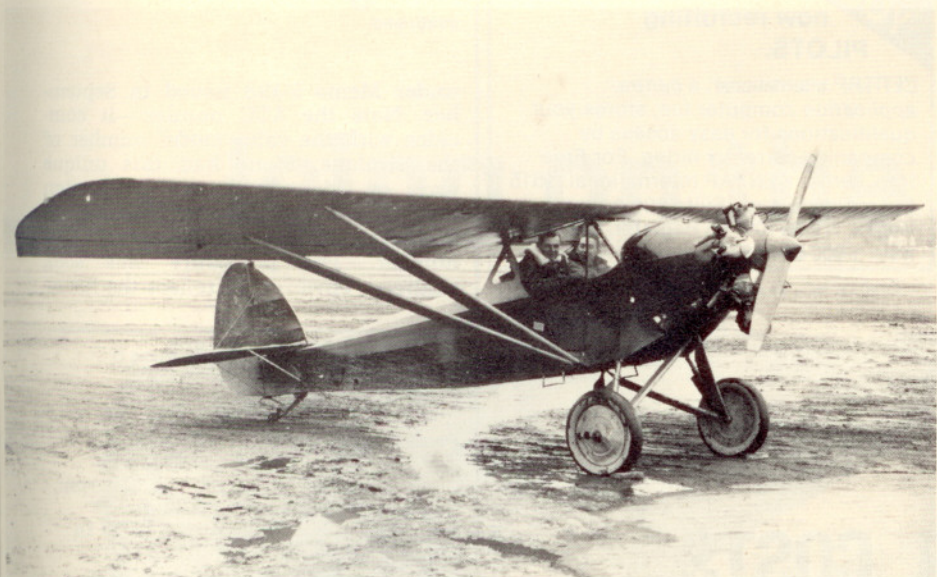
A later Monoprep had a revised tail shape and different landing gear but retained the original curved windshield. A full-depth, hinge-forward door on each side of the cockpit has a step below it.
